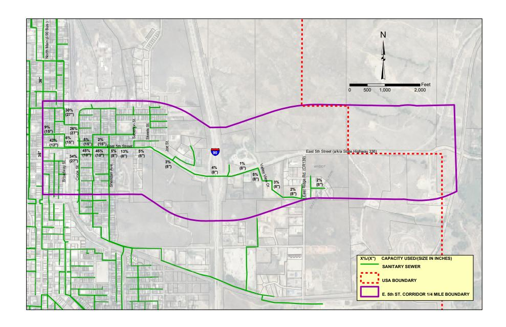
Figure 8. Sewer capacity map
