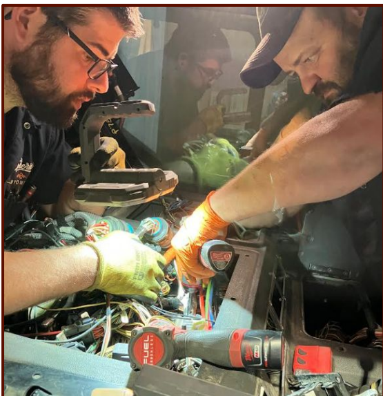
Erik and Rod diagnosing a transmission wiring issue.
