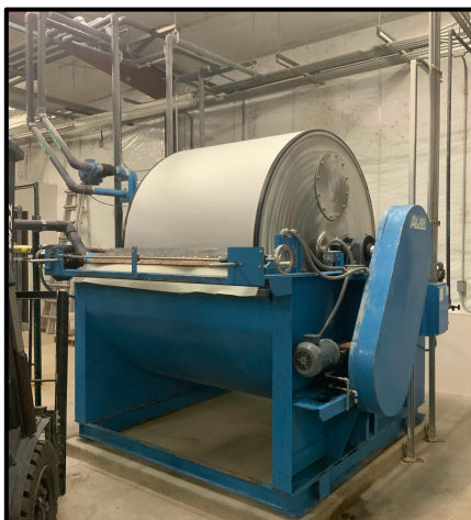
ALAR System at the plant used to remove FOG.
